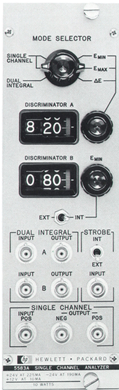
Fig. 1. New single-channel nuclear pulse-height analyzer (HP Model 5583A) with 200 nanosecond multiple pulse resolution.
